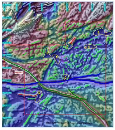
Figure 1. Structural Interpretation on aeromagnetic image (RTP NW shade with 2VD AGC transparency)
