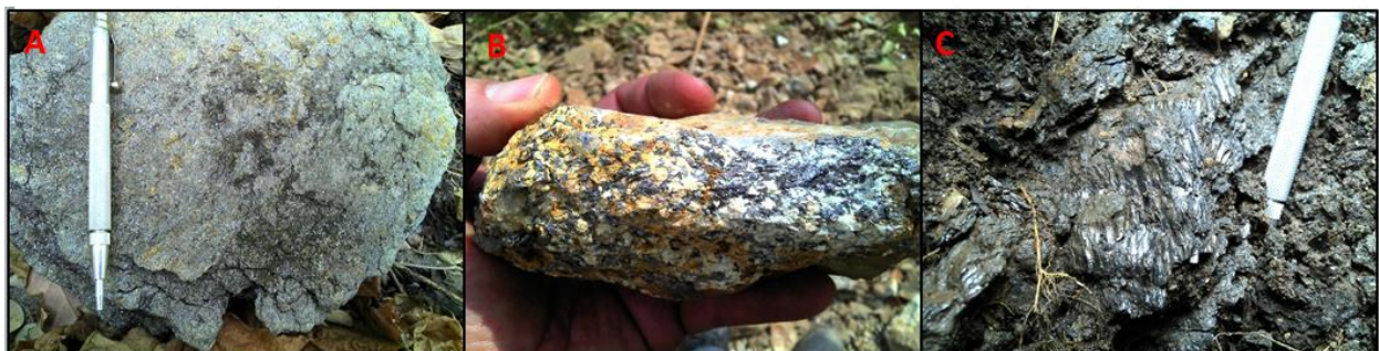
Figure 5. Three main varieties of graphite mineralisation at Nachingwea. A - graphite-quartzite, B - graphite-gneiss and C - semi massive graphite schist
